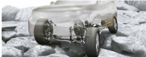
KDSS\* - This super-advanced system allows your suspension to adjust and dynamically respond to the landscape, giving you more robust traction, enhanced stability, steering response, comfort and unmatched off-road control. This is the smoothest off-road drive you'll ever have.
